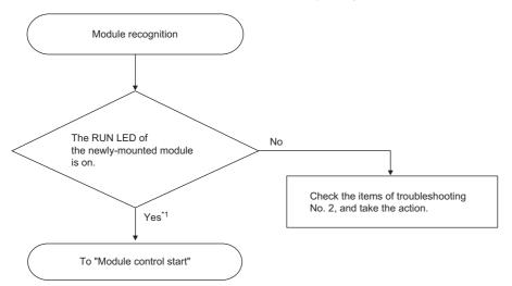
\*1 When the initial setting is configured with the module parameter of an engineering tool, the setting of the module parameter is applied when the RUN LED turns on.
