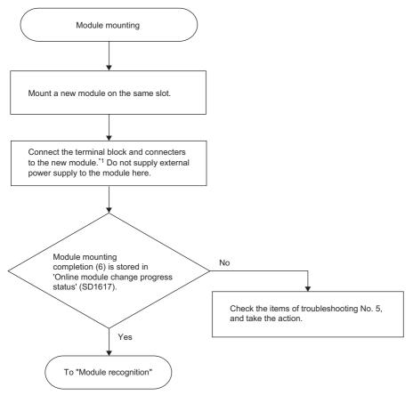
\*1 Insert the SD memory card (which was removed when the module was removed) to a new module, if MES interface module, high speed data logger module, C intelligent function module, and OPC UA server module are used.
